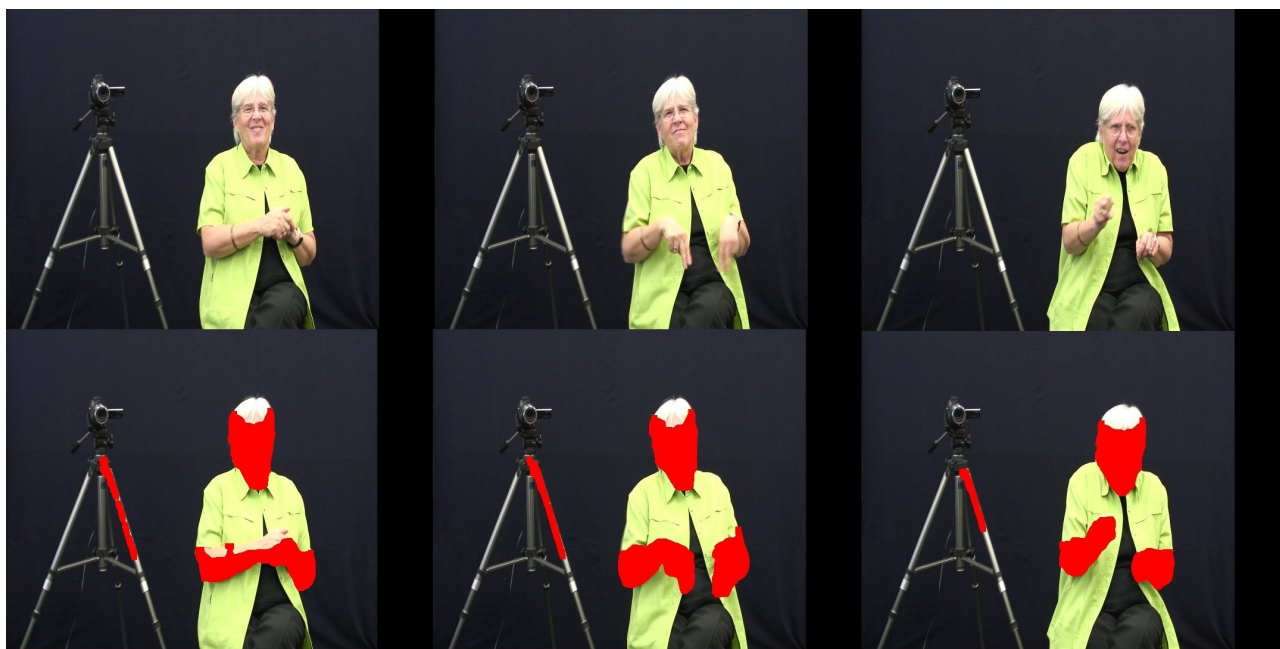
Fig.3. Skin segmentation segmentation: Areas in the image correspond to moving parts of the body which color is similar to that of skin, such face, arms, and hands.
