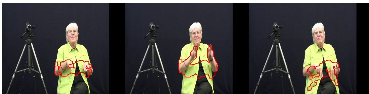
Fig.2. Background/foreground segmentation: Areas in the image with motion appear segmented. These regions may belong both to the signer's limbs and to body parts.
